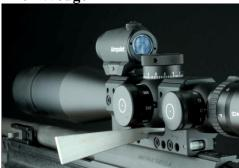
The rotation of the scope is extremely important on a long range gun. We have a mechanical solution to take care of the problem: a simple 10-degree "wedge" that is inserted into a 10-degree slot in the mount when the scope is being mounted. This simple tool will guarantee that the scope is level. It works against the flat underside of the scope, which on quality scopes is indexed to both the reticle and the turrets' movements.
