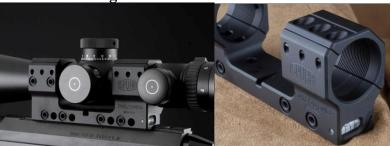
The mount is machined in one piece from a solid billet. The material used is Aluminum 7075, which is one of the strongest aluminum grades available. The strength is better than lower grades of steel. The reason we have chosen to use aluminum is it's price, low weight and strength.
